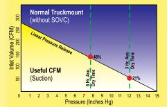
The chart to the right illustrates the effect of replacing the spring and disc valve with an S.O.V.C. digitally controlled valve. PowerPlus calibrates each S.O.V.C. unit to open the pressure relief valve at the customers specified pressure. The result is maximum suction while ensuring maximum safety.
