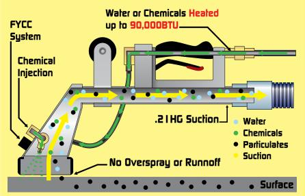
**WHAT IS CLEAN AND CAPTURE?** Clean and Capture is a proprietary technology of PowerPlus Professional Cleaning Solutions that utilizes heat, suction, pressure, and chemical properties to achieve a decontamination solution second to none. The PRODIGY BIO is completely integrated with this system that can provide a safe, inexpensive, way to reclaim contaminated areas.
